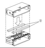
1 Engage the catch pins on the removal tool and remove the two locks on the lower level.
